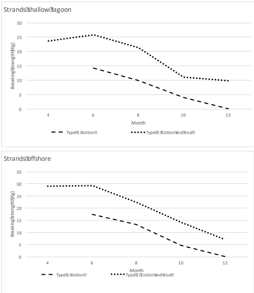
**Figure 4.** Biodegradable ropes' strands degradation with time. For those anchored in offshore waters (bottom) and within the lagoon (top)
