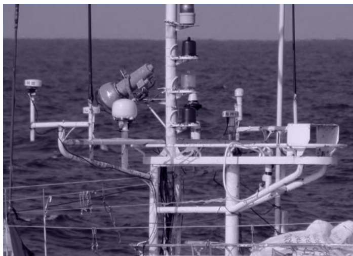
Roof of the bridge of a tuna longliner where the antenna of VMS is commonly installed
