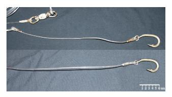
Fig. 2. The wire (above) and nylon (below) leaders used in the study. Also shown is a weighted swivel.
