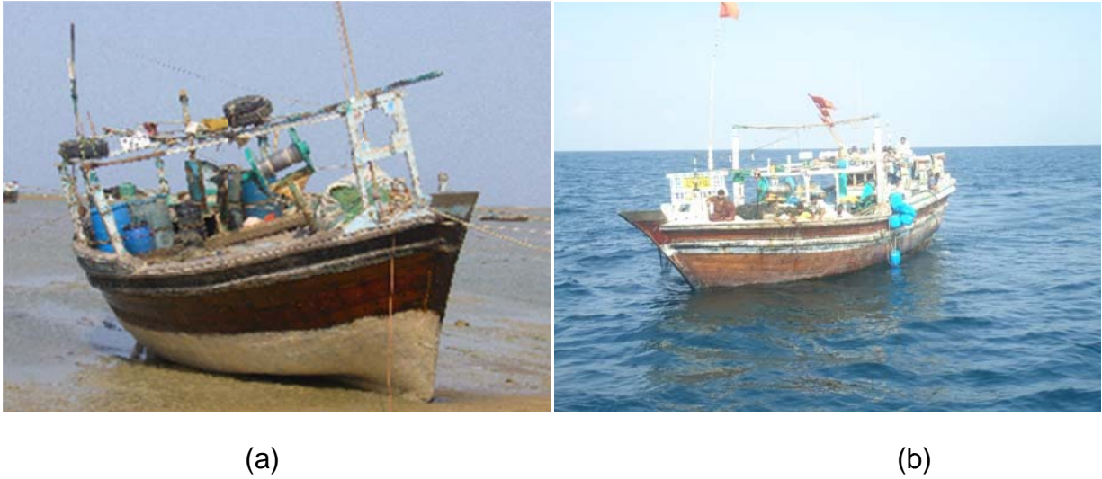
Fig. 1. Gillnet fishing boats (a) Smaller Tuna Gillnetter ('hora'/'rachin') (b) Large Tuna Gillnetter
