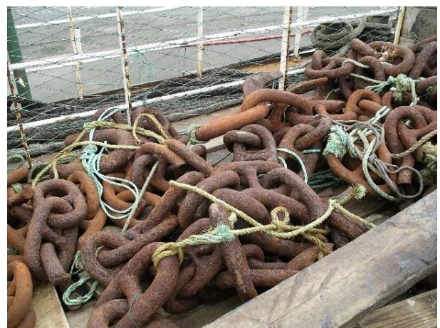
Chain links used to anchor the net.
