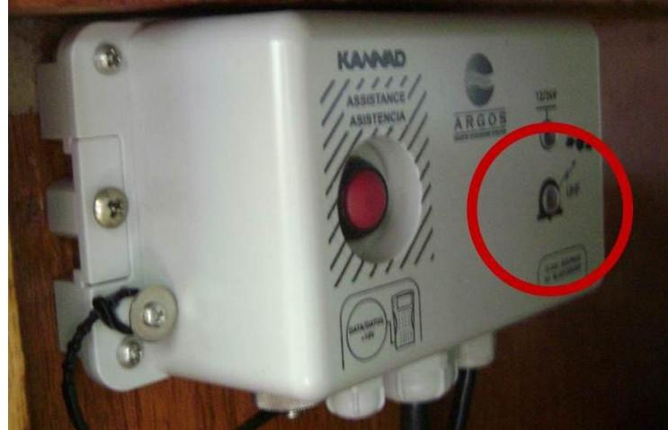
**Figure 30:** Argos junction box switched off.
