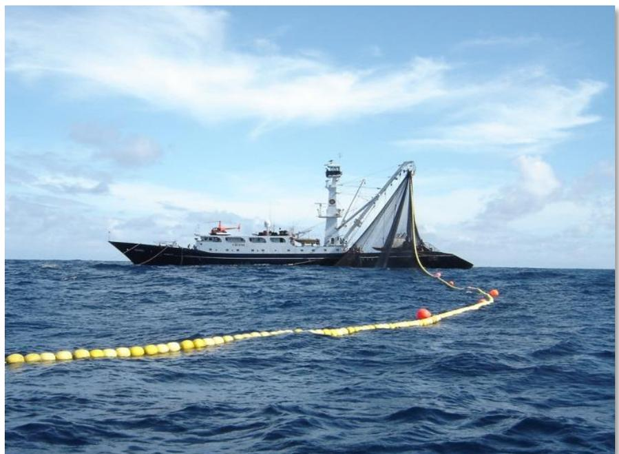
**Figure 15:** Oceanic tuna seiner in fishing operation in the Indian Ocean.
