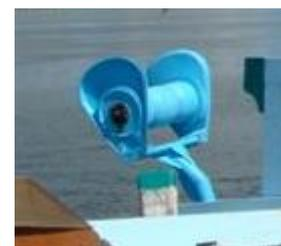
**Figure 18:** Roller / guide used on tuna gillnet vessels.
