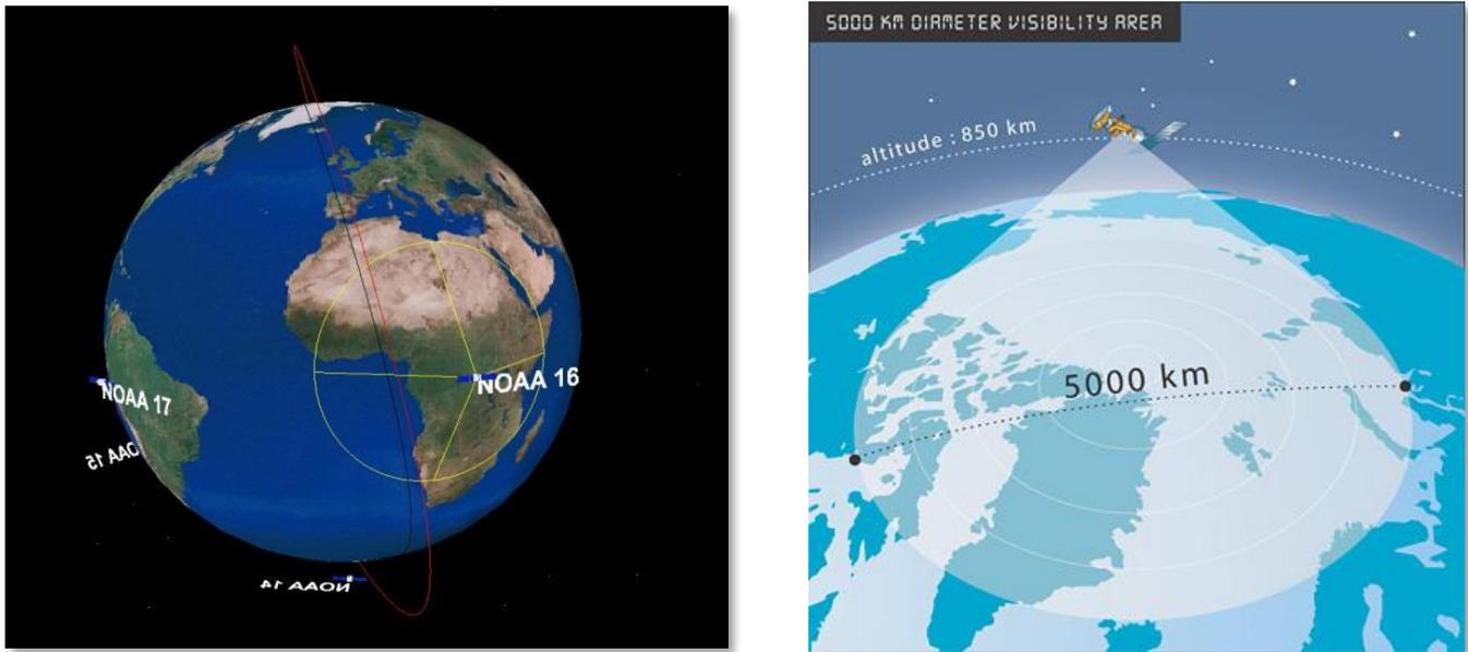
**Figure 19:** Argos satellites constellation and coverage.
