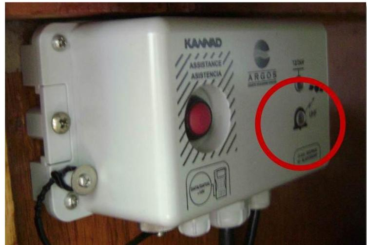
**Figure 30:** Argos junction box switched off.
