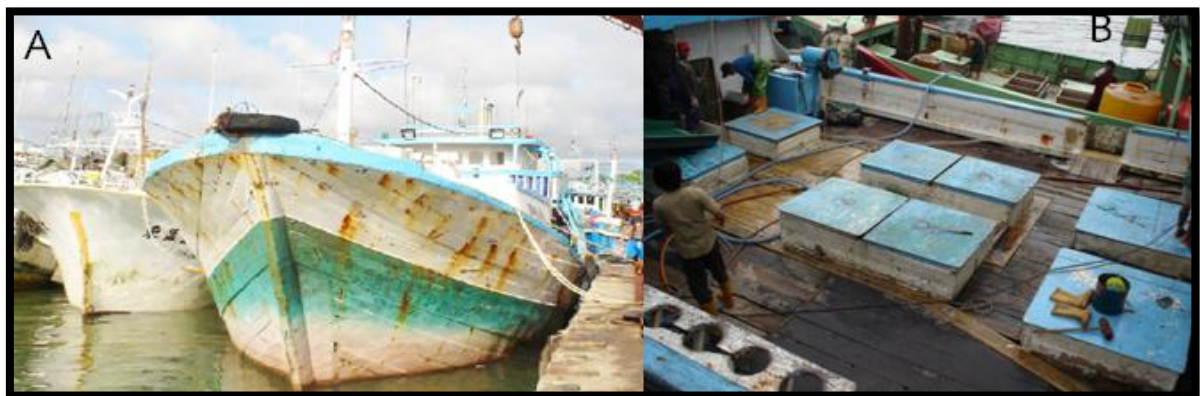
Figure 2 Wood tuna longliners (A) an overview and (B) fish storage rooms
