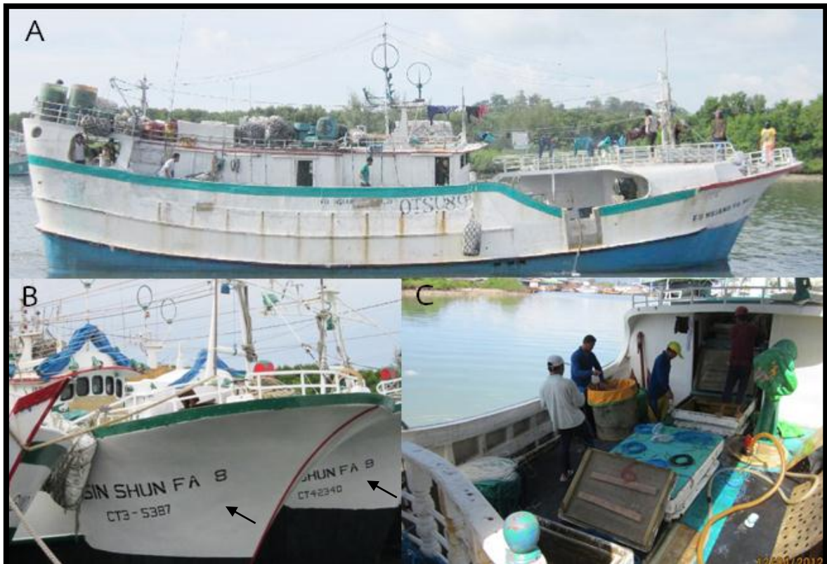
Figure 1 Wood-fiberglass tuna longliners (A) an overview, (B) registration number and (C) fish storage rooms
