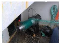
Drum or net roller used to haul in the gillnet
