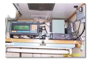
Figure 27: Two VMS units installed onboard a tuna longliner.
