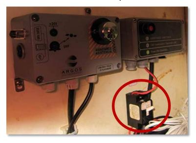
Figure 29: Argos junction box with on/off switch.
