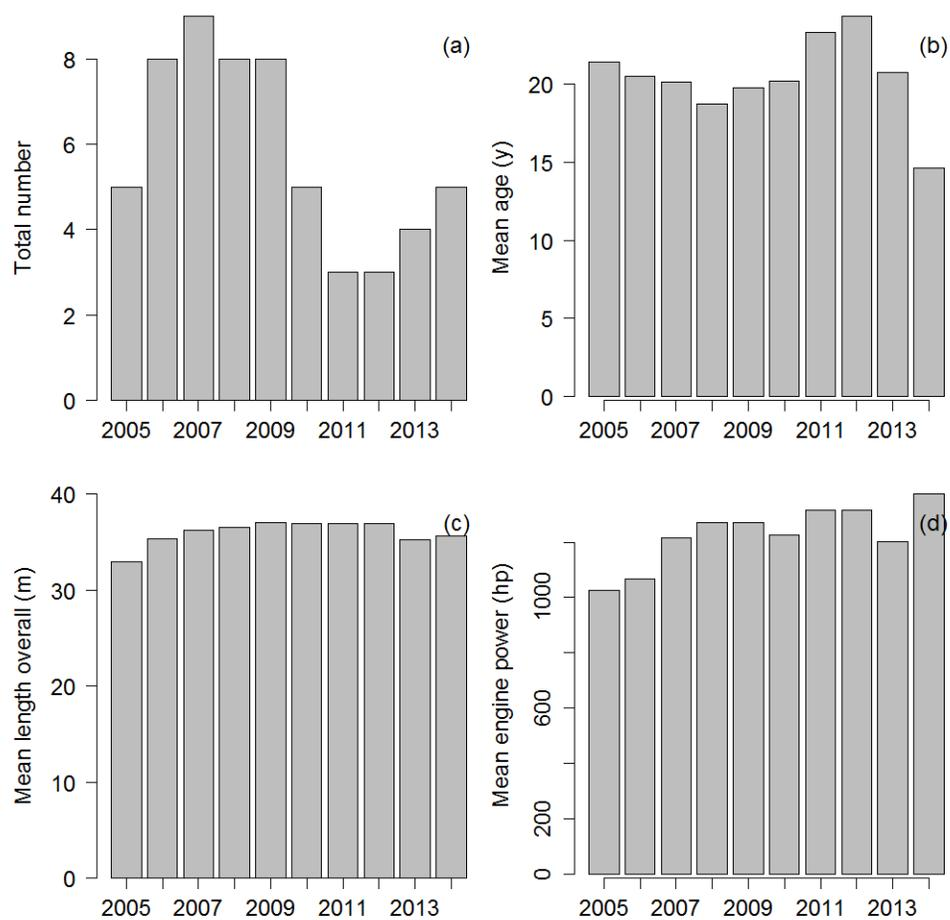
**Fig. 1.** Yearly main characteristics of the Seychelles support vessel fleet during 2005-2014: (a) Total number of vessels in operation, (b) Mean age of the vessels, (c) Mean length overall, (d) Mean engine power
