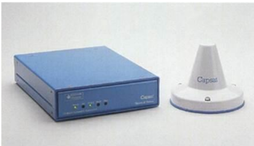
Figure 23: Capsat Unit and antenna.
