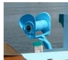
Figure 18: Roller / guide used on tuna gillnet vessels.
