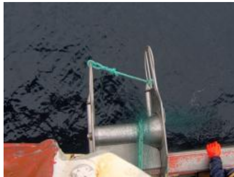
Guide to haul a gillnet over the side inboard.
