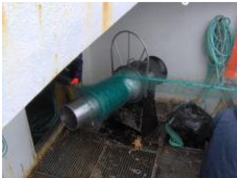
Drum or net roller used to haul in the gillnet
