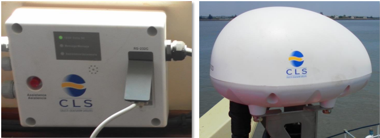
Figure 28: Junction box (left) and dome (right) of a Thorium unit.
