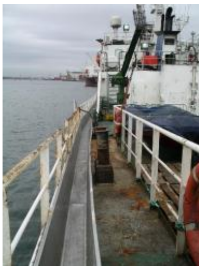
Chute or channel used to guides the net from the hauling point to the stern where it is stored ready for deploying.
