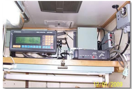
Figure 27: Two VMS units installed on-board a tuna longliner.
