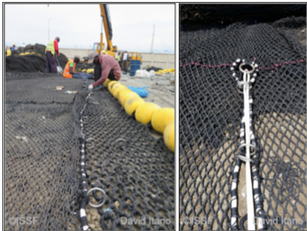
Figure 9.1. Construction of the top portion of the release panel (left) and detail of rings at the bottom corner (right).
