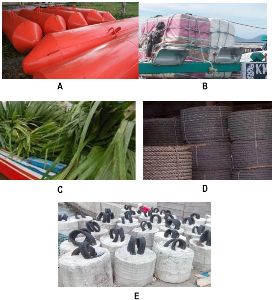
Figure 3. Construction materials common to FADs in western Indonesia: (A) steel pontoon, (B) polystyrene block (gabus), (C) subsurface attractor nypa leaf, (D) polypropylene main rope , and (E) concrete anchor blocks (photos : Proctor and Widodo).
