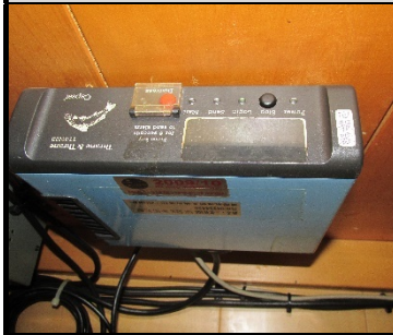
10. Thrane & Thrane (Sailor) Capsat 6194 terminal control unit TT3027D Antennae
