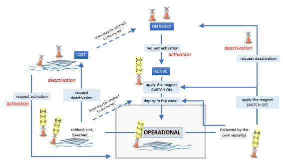
Figure 1. Life cycle of an instrumented buoy
