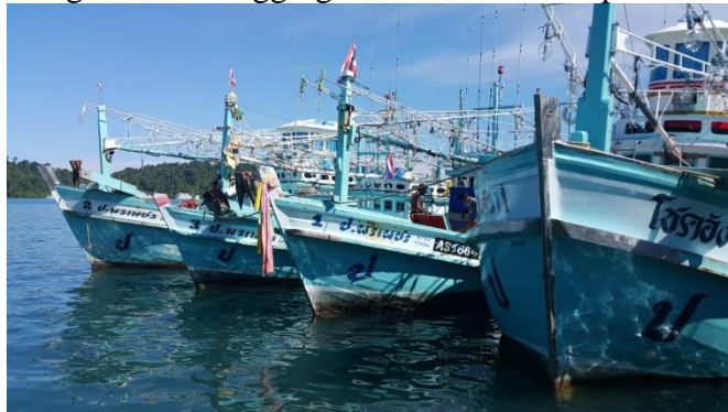
Figure 3 Light luring vessel for aggregated fish school of purse seines.
