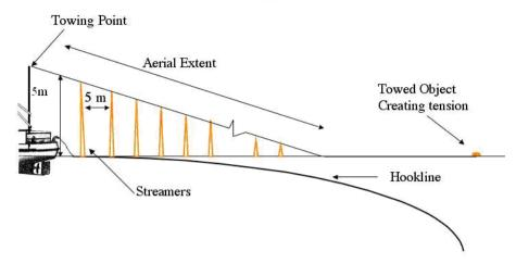
Figure 1. Diagram of Bird Scaring Streamer Line.
