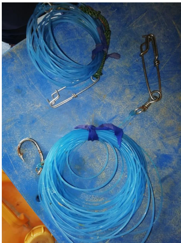
Fig. 3. Branch line stored on board for experimental longline
