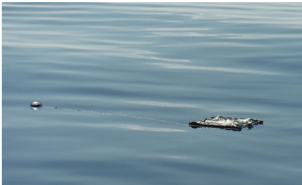
Fig. 1. Example of drifting human-made Fish Aggregating Device and its associated instrumented buoy (©ORTHONGEL-IRD/Yannick Baidai)
