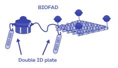
Drawing of the procedure to attach the BIOFAD ID number shown in the metallic plate to the raft and associated echo-sounder buoy.
