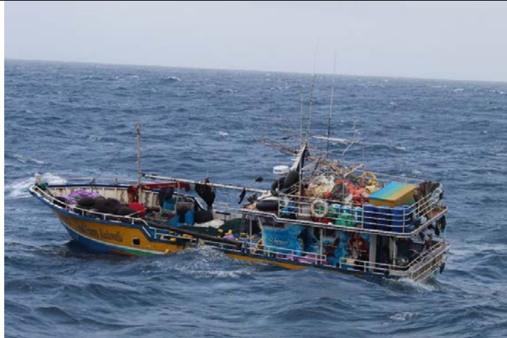
Figure 1. Port aspect of the vessel. Foredeck visible with gill nets on deck and slightly hanging over the gunnel. LL barrels and hooks shown on mid deck.
