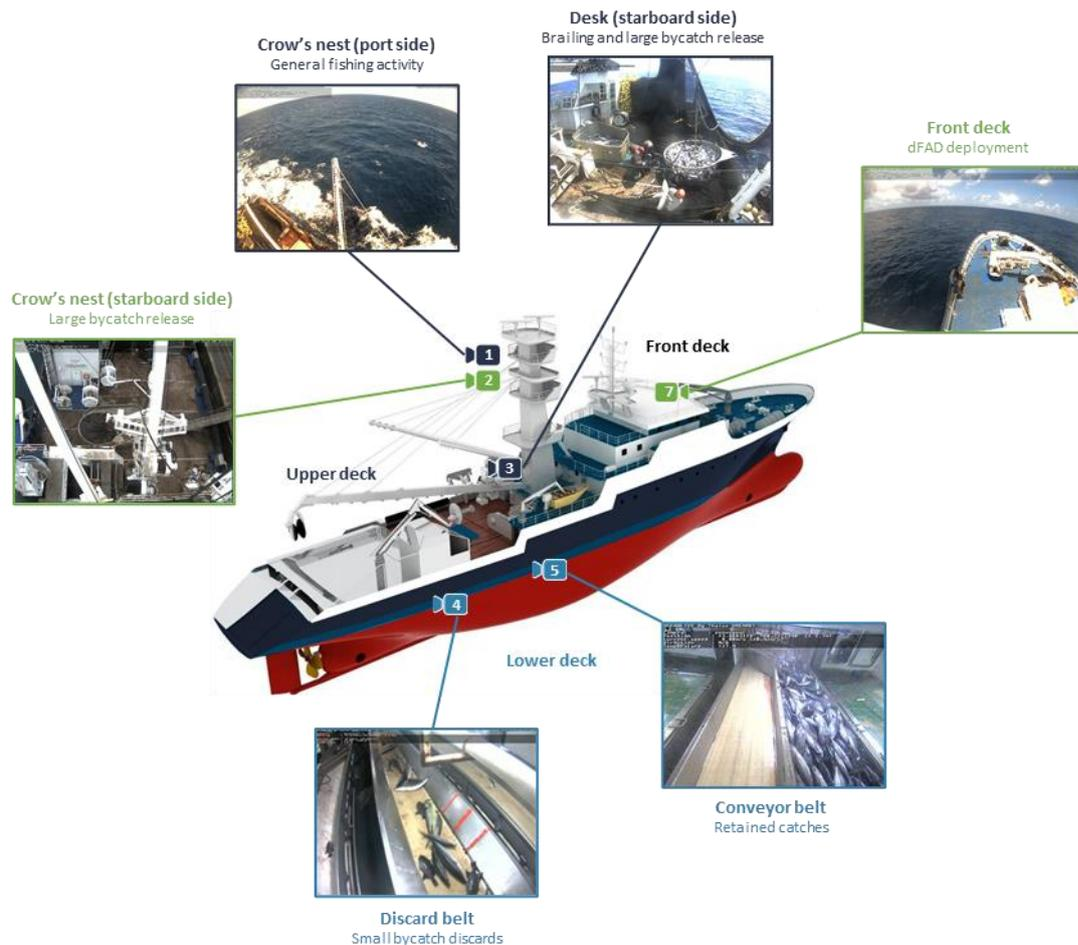
**Figure 3** : EMS configuration 2.0, currently in deployment. Additional cameras (starboard side crow's nest and front deck) are highlighted in green.
