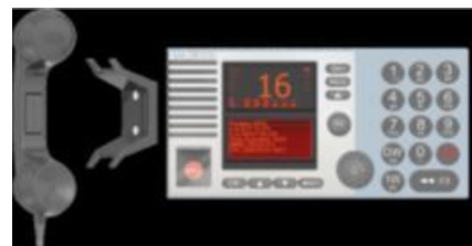
VHF DSC transmitter-receiver metric wave (range: about 20 miles)
