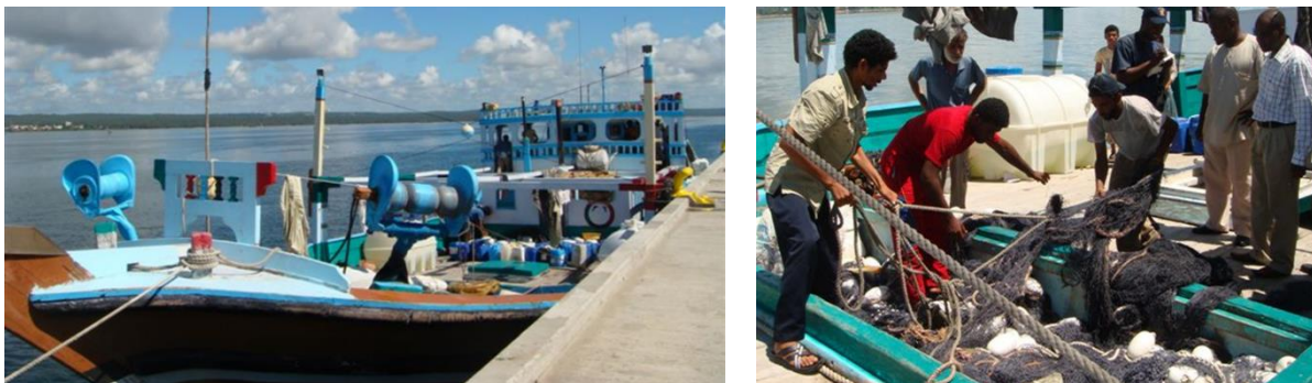
Figure 33: Hydraulic drums on a gillnet vessel in the Indian ocean and nets stored in hold below deck.
