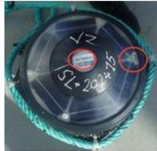
Figure 12 – Marked satellite buoy. Manufacturer unique identification code is identified with red ovals. White codes painted on the buoy are the identification codes added by buoy owner (© AZTI Tecnalia).
