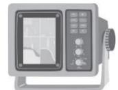
**48. Sonar:** The sonar displays solid objects in the water column below or to the side of the vessel. It can display the presence and movements of fish close to the vessel. This includes bait fish and rainbow runners, as well as tuna. The sonar is a critical piece of equipment when a vessel is preparing to make a set and wants to keep an eye on the school of fish. The size, depth, speed and the total tonnage of the school of tuna can be judged from the sonar display.
