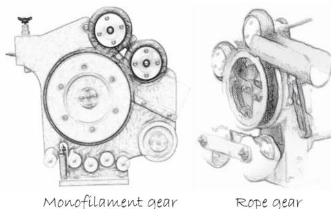
**2. Line hauler:** The line hauler uses hydraulic motor to assist with retrieving the main line. There are different types of mainline haulers. Traditional rope haulers, Japanese reel system, Monofilament reel system, etc. The line hauler is used predominantly on vessels that use a multi-strand rope or braided monofilament nylon mainline, which is stored in layers in a large bin; storage well or reel. The line hauler is generally positioned on the starboard side.
