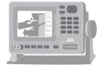
**47. Depth Sounder:** The depth sounder searches for and displays objects below the vessel. It may show the presence of fish and can be used to help with navigation, especially when travelling in shallow waters or entering harbour areas.
