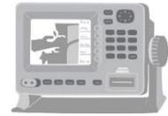
**47. Depth Sounder:** The depth sounder searches for and displays objects below the vessel. It may show the presence of fish and can be used to help with navigation, especially when travelling in shallow waters or entering harbour areas.
