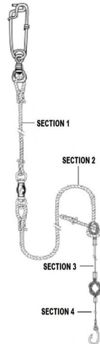
**9. Branchline section diameter:** Measure the diameter of each branch line section preferably *in millimetres (mm)* with a calliper or place the mainline against a ruler to read off line width. *Measure at least every single branchline in one 'basket'.* The value can be recorded up to one decimal place.
