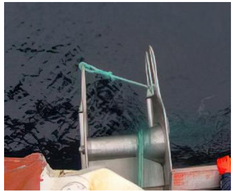
Guide to haul a gillnet over the side inboard.
