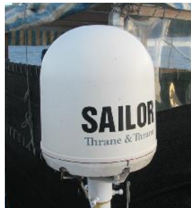
Figure 59: Cobham/SAILOR 250 FLEET BROADBAND unit and antenna
