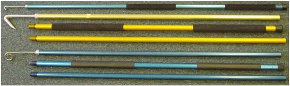
Figure 89: Long handled device (from top): J-Style de-hooker, line cutter and de-hooker for ingested hooks
