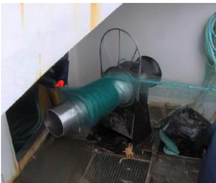
Drum or net roller used to haul in the gillnet
