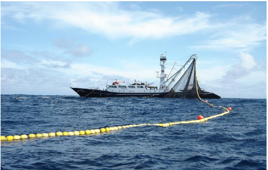
Figure 35: Oceanic tuna seiner in fishing operation in the Indian Ocean
