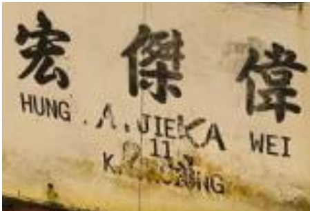
Figure 83: Confused marks on the stern of a longliner that need further investigation during the inspection
