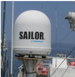
Figure 59: Cobham/SAILOR 250 FLEET BROADBAND unit and antenna
