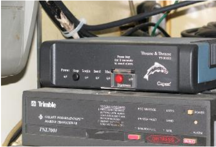
Figure 63: Two VMS units installed on board a tuna longliner (Thrane & Thrane 3022D INMARSAT and Junction Box of the Trimble Galaxy unit)
