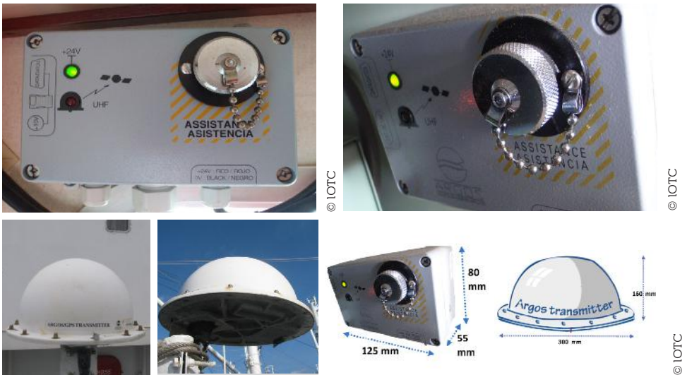
Figure 49: MARGE unit and antenna
