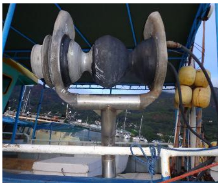
Figure 38: Roller / guide used on tuna gillnet vessels
