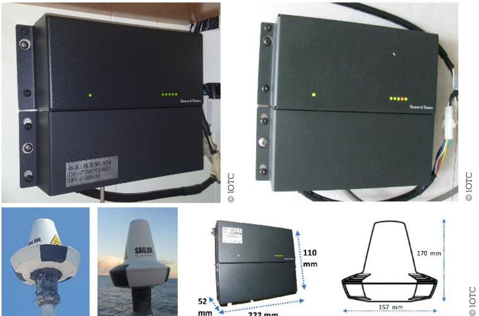
Figure 57: Thrane & Thrane (Sailor) Capsat 6194 terminal unit and antenna
