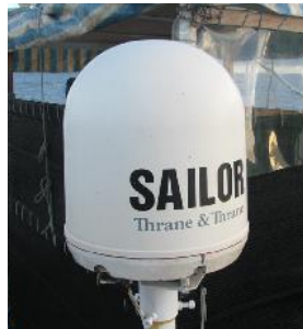
Figure 59: Unité et antenne Cobham/SAILOR 250 FLEET BROADBAND
