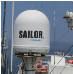
Figure 59: Unité et antenne Cobham/SAILOR 250 FLEET BROADBAND
