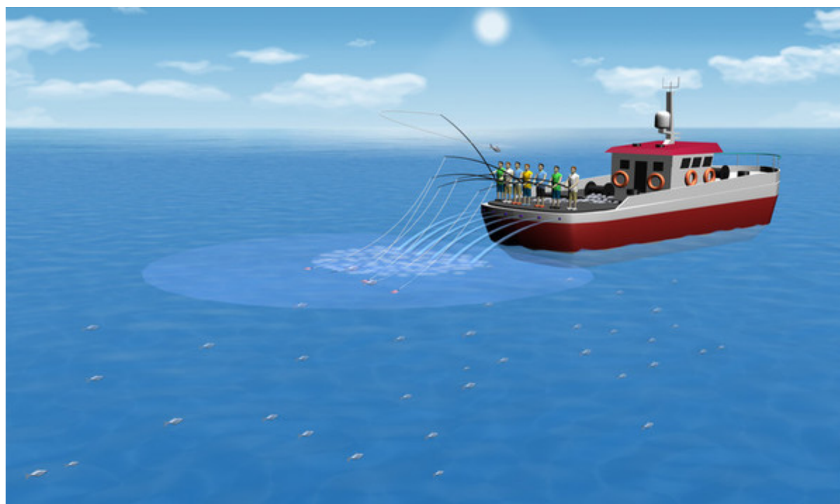
Figure 5. Hand-operated pole-and-lines (LHP 09.1) fishing for skipjack tuna ( Katsuwonus pelamis ) with live bait chum and water jets. Water jets come from the stern of the boat (underneath the fishers)
