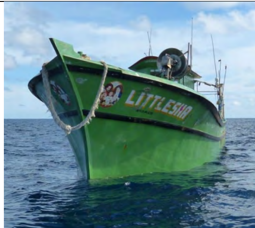
[Fig.8] Port bow detail: mounted net hauler and deployment ready dan-buoys.
