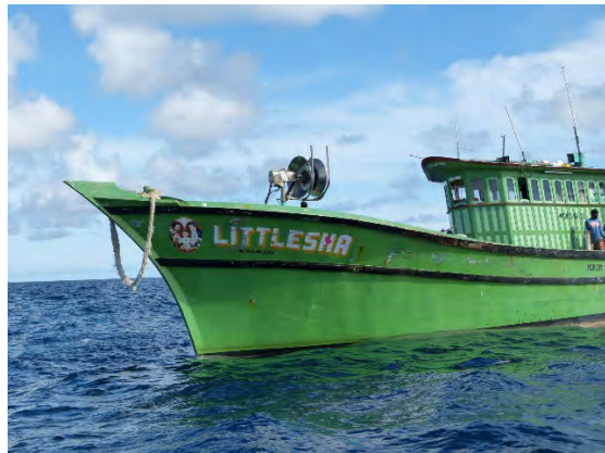
[Fig.9] Port bow and mounted line hauler.
