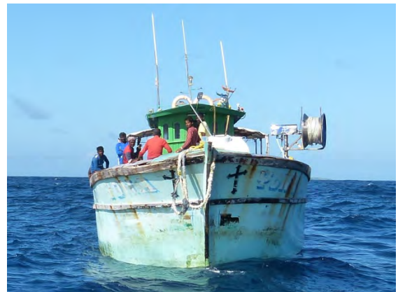
[Fig.12] Yona bow. Gill net winch is mounted.
