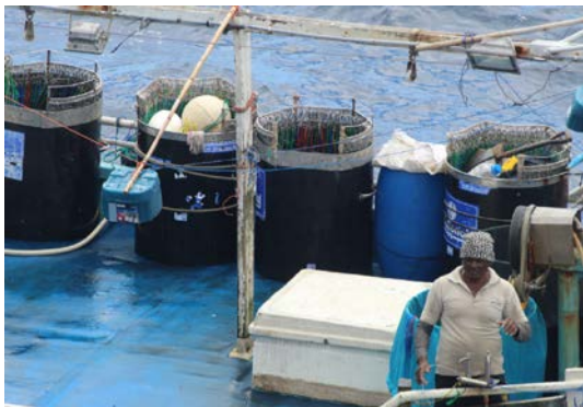
[Fig 9] Line guide on rail & auto hauler behind crewman. Long-line barrels along port rail.
