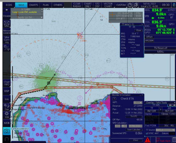
[Fig.1] Initial position of radar targets and BPV when targets fixed ~10nm North of Peros Banhos on BPV ECDIS (14/02/22 09:30).
