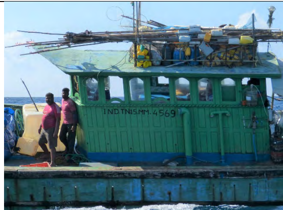
[Fig.14]Port: ID many floats and dan-buoys stowed on roof
