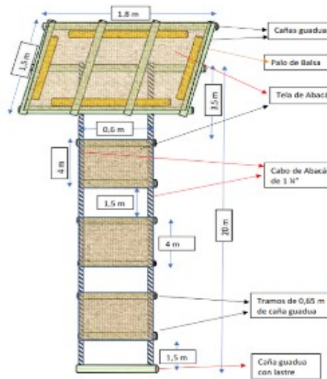
Figure 1. Non-Entangling biodegradable dFAD design (c) TUNACONS
