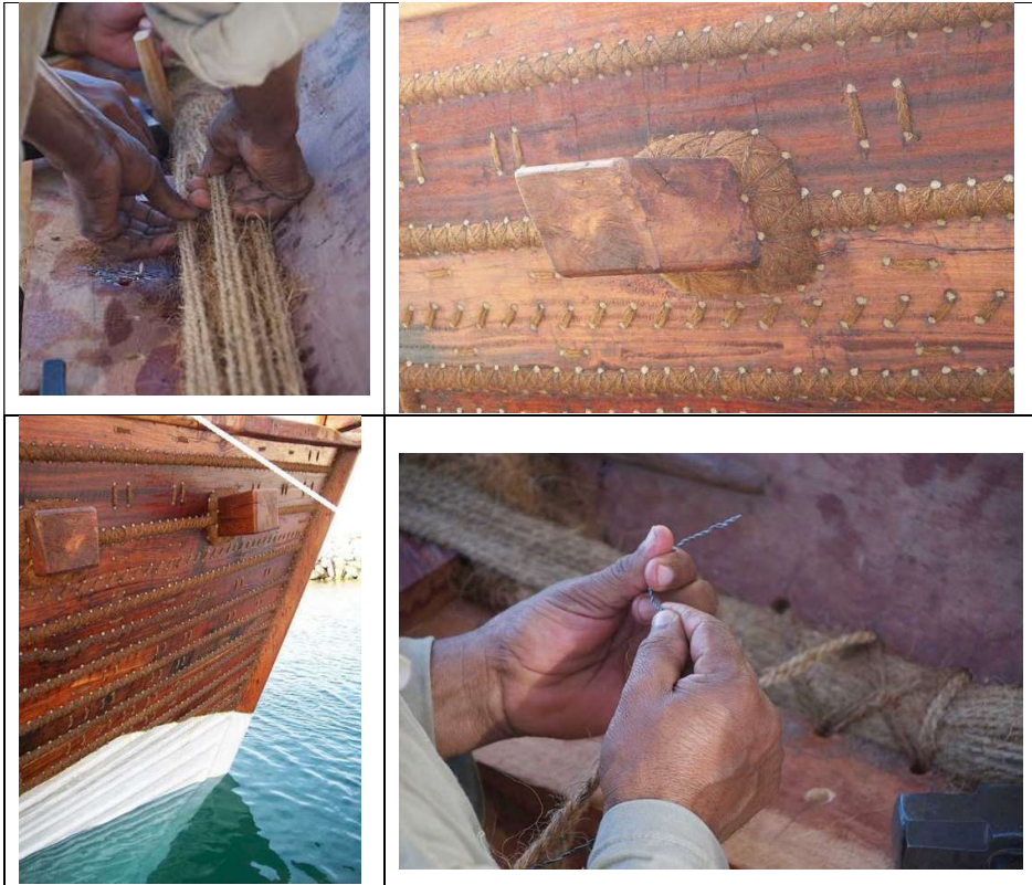
Figure 4. Traditional ‘sewn’ boats from Oman were built by using coir coconut fibre rope to bind planks together. The biodegradable rope used in this type of construction were in constant contact with seawater and lasted a lifetime.
