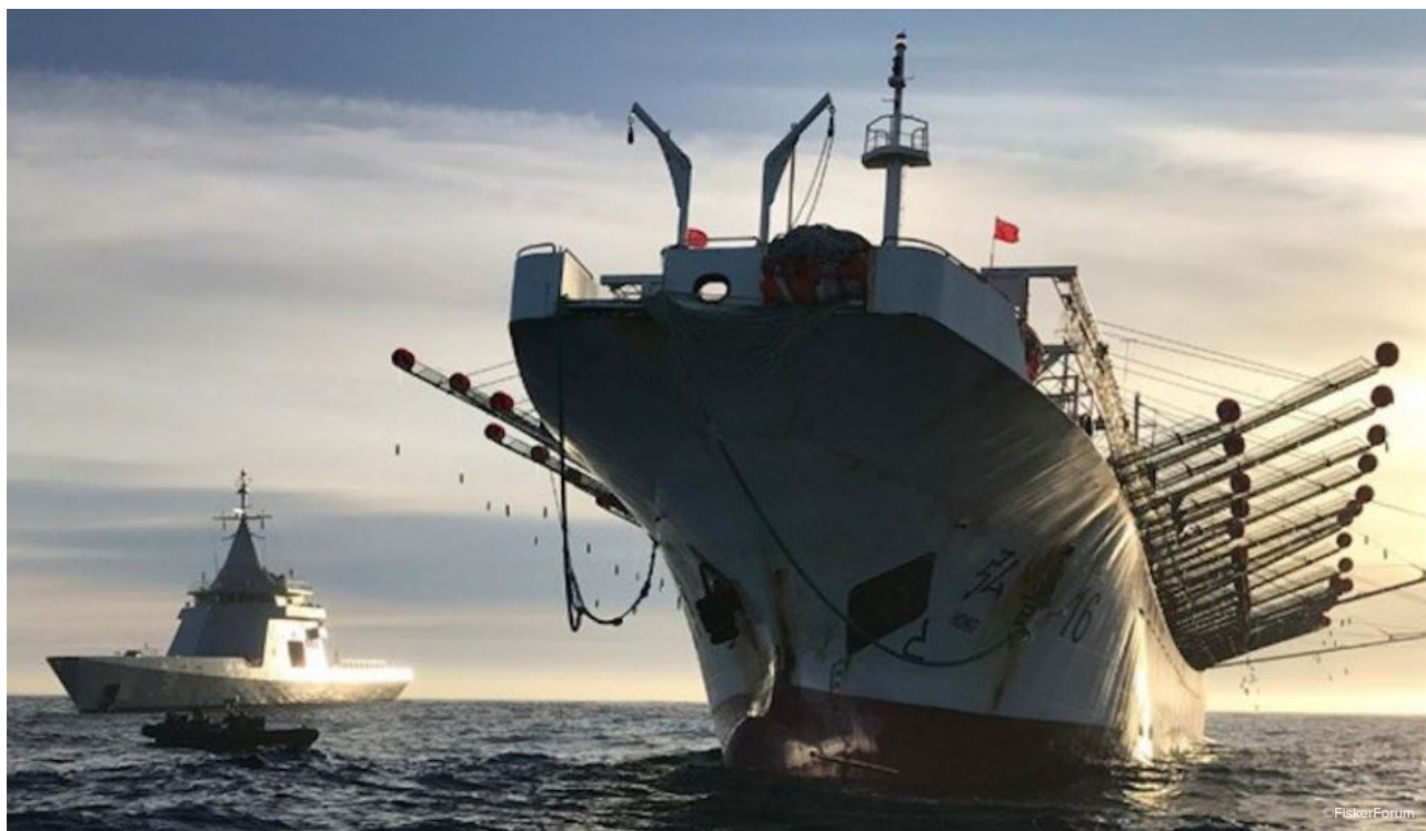
Image of a squid vessel with jiggering machines visible on each deck side – note that this image was taken in the Southwest Atlantic. Whilst AIS indicates that vessels reported to be jiggers do operate in the NWIO, none were physically sighted in the area in May 2021.
