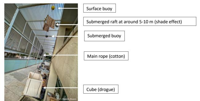
Figure 2. The JellyFAD mounted at ICM facilities.
