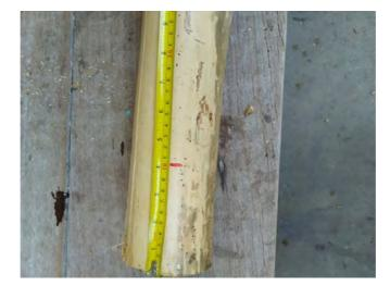
2. Measure 10cm from both ends of the bamboo cane and mark
