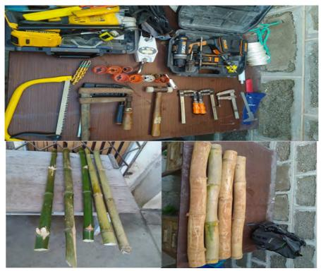
Figure 1. Tools and bamboo canes (1.35 cm) needed to build the biodegradable FAD.
