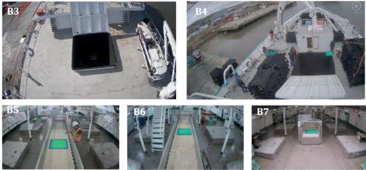
Figure 1. (A) 6-cameras EM system installed in a purse seine covering main areas of fishing and fish handling operations (from Murua et al., 2020b) and (B) 7-cameras EM system (4 in the upper deck and 3 in the well deck) installed in a purse seine covering main areas of fishing and fishing handling operations including 1 more camera in the conveyor belt: (B1) 360° Panoramic view camera (e.g port side view), (B2) Crews nest stern view camera, (B3) Working deck crane camera view, (B4) Foredeck view camera, (B5) Conveyor belt stern camera view, (B6) Conveyor belt middle camera, and (B7) Conveyor belt bow camera (source: Digital Observer Services).
