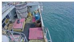
Figure 2. 3-cameras EM equipment installed on a longline covering main areas of fishing and fish handling operations. View of the 3 cameras: (left panel) Stern camera - setting longline providing information on hooks, floats, mitigation techniques and bait; (middle panel) Fishing deck 1 - hauling information, captures and discards, species ID, size and fate; and (right panel) Fishing deck 2 - fate of the species, size, species ID (source: Digital Observer Services).
