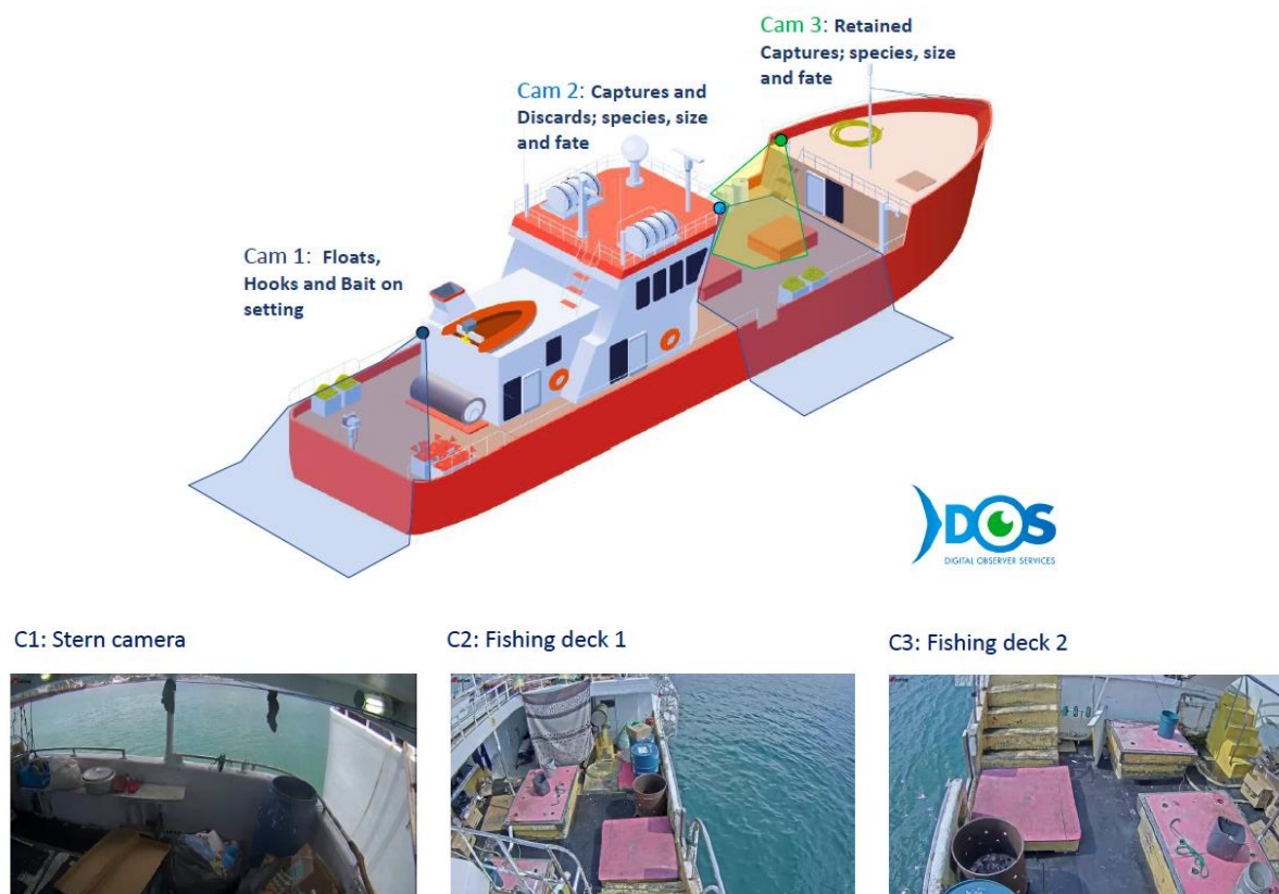
Figure 2. 3-cameras EM equipment installed on a longline covering main areas of fishing and fish handling operations. View of the 3 cameras: (left panel) Stern camera - setting longline providing information on hooks, floats, mitigation techniques and bait; (middle panel) Fishing deck 1 - hauling information, captures and discards, species ID, size and fate; and (right panel) Fishing deck 2 - fate of the species, size, species ID (source: Digital Observer Services).
