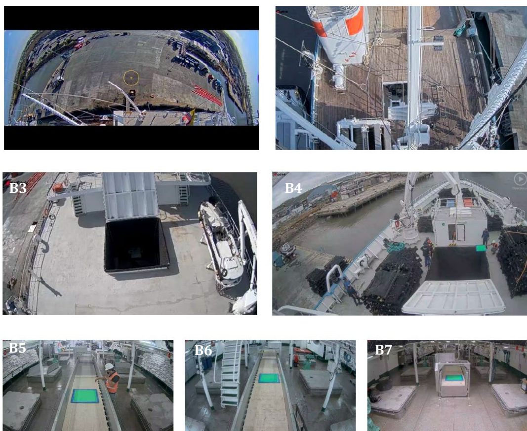
Figure 1. (A) An example of a 6-camera EM system installed in a purse seine covering main areas of fishing and fish handling operations (from Murua et al., 2020b) and (B) 7-camera EM system (4 in the upper deck and 3 in the well deck) installed in a purse seine covering main areas of fishing and fishing handling operations including 1 more camera in the conveyor belt: (B1) 360° Panoramic view camera (e.g port side view), (B2) Crows nest stern view camera, (B3) Working deck crane camera view, (B4) Foredeck view camera, (B5) Conveyor belt stern camera view, (B6) Conveyor belt middle camera, and (B7) Conveyor belt bow camera (source: Digital Observer Services).
