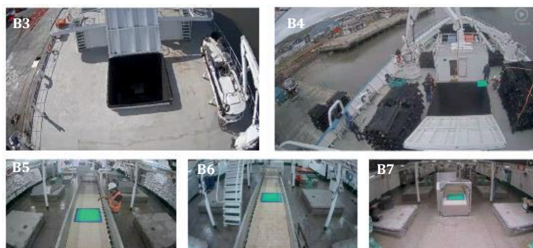
Figure 1. (A) 6-camera EM system installed in a purse seine covering main areas of fishing and fish handling operations (from Murua et al., 2020b) and (B) 7-camera EM system (4 in the upper deck and 3 in the well deck) installed in a purse seine covering main areas of fishing and fishing handling operations including 1 more camera in the conveyor belt: (B1) 360° Panoramic view camera (e.g port side view), (B2) Crows nest stern view camera, (B3) Working deck crane camera view, (B4) Foredeck view camera, (B5) Conveyor belt stern camera view, (B6) Conveyor belt middle camera, and (B7) Conveyor belt bow camera (source: Digital Observer Services).
