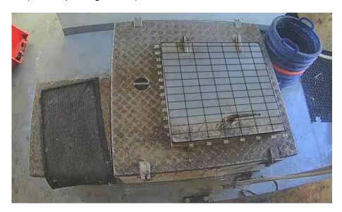
**Fig. 1**: Example of a calibrated hatch onboard a commercial fishing vessel. These areas will vary from vessel to vessel, depending on available surfaces and the species being measured. This image is provided as an example from a non-tuna fishery. For tuna and tuna-like fisheries, the defined areas will have to be larger to accommodate larger species.
