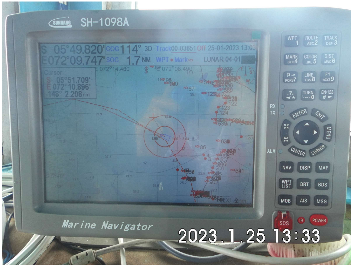
[Fig.4] Second GPS / AIS combination unit with gear deployments marked
