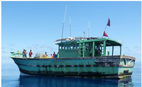
[Fig.13] Port. Buoys on wheelhouse roof but floats on deck. Note fishing light mounted off wheelhouse ladder.
