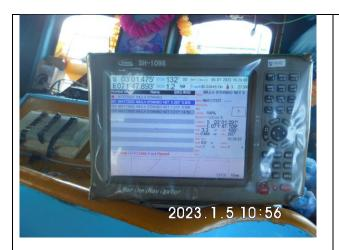
[Fig 21.] Vessel GPS (Z + 5:30) and bearing and distances to line buoys.
