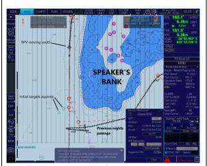
[Fig.3] 15:31 targets identified on ECDIS
