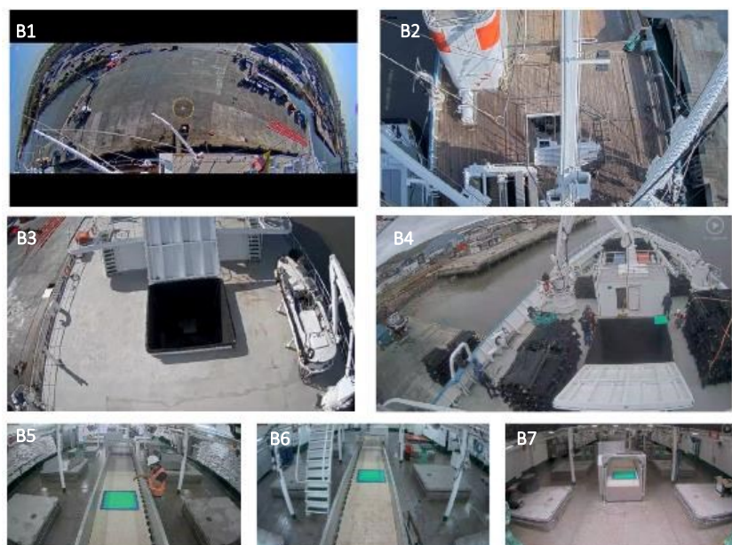
Figure 1. (A) An example of a 6-cameras EM system installed in a purse seine covering main areas of fishing and fish handling operations (from Murua et al., 2020b) and (B) 7-cameras EM system (4 in the upper deck and 3 in the well deck) installed in a purse seine covering main areas of fishing and fishing handling operations including 1 more camera in the conveyor belt: (B1) 360° Panoramic view camera (e.g port side view), (B2) Crow's nest stern view camera, (B3) Working deck crane camera view, (B4) Foredeck view camera, (B5) Conveyor belt stern camera view, (B6) Conveyor belt middle camera, and (B7) Conveyor belt bow camera (source: Digital Observer Services).
