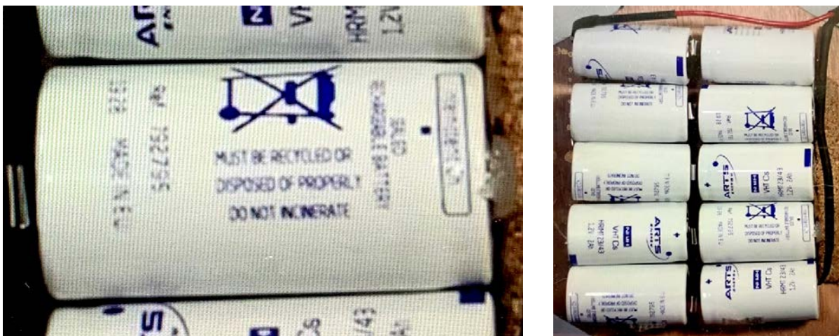
Figure 4 – Nickel metal hydride (NiMh) batteries recovered from a Marine Instruments drifting FAD satellite beacon in the Indian Ocean displaying the WEEE logo that calls for proper recycling of hazardous waste. PHOTO CREDIT: COPYRIGHT ALEX HOFFORD
