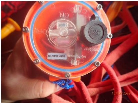
[Fig. 20] Skynav AT-102 AIS GPS tracker, ref number SHO98509149.
