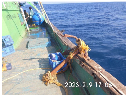
[Fig.18] Anchor not stowed
