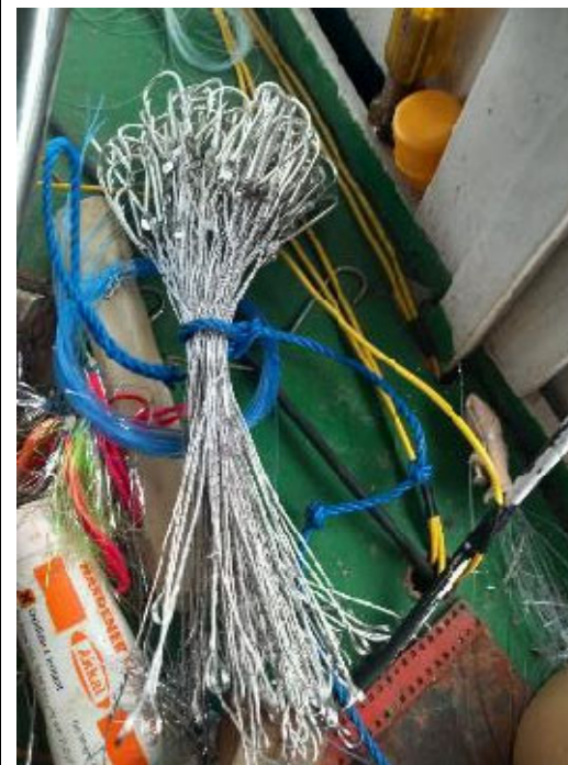
[Fig. 22] Wire trace with hooks attached
