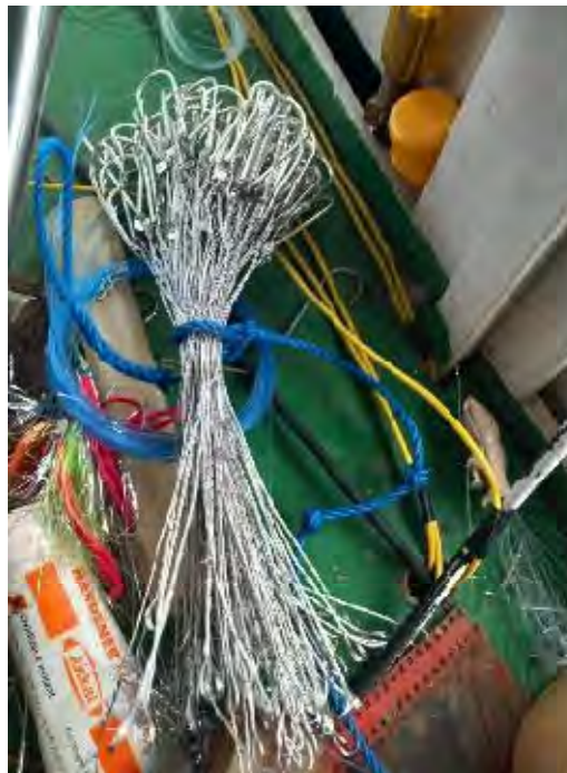
[Fig. 22] Wire trace with hooks attached
