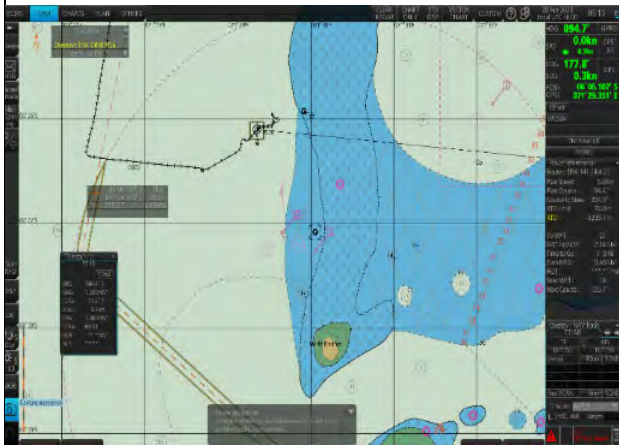
[Fig. 9] ECDIS. During boarding.
