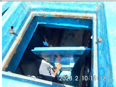
[Fig.22] Checking internal panel between iced holds.
