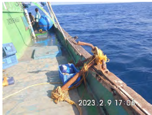
[Fig.18] Anchor not stowed
