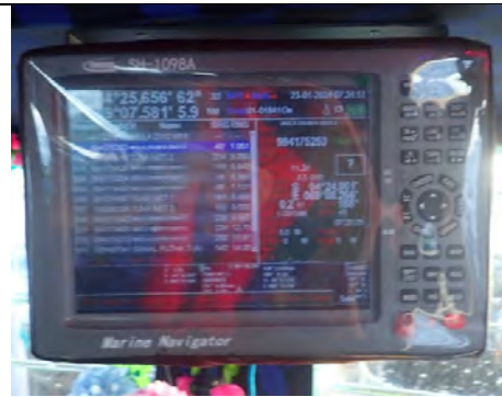
[Fig.8].GPS with list of the AIS marker buoys in the water
