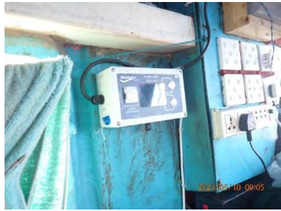
[Fig 39] BlueTraker VMS Communications ConBox 2018 LCD.
