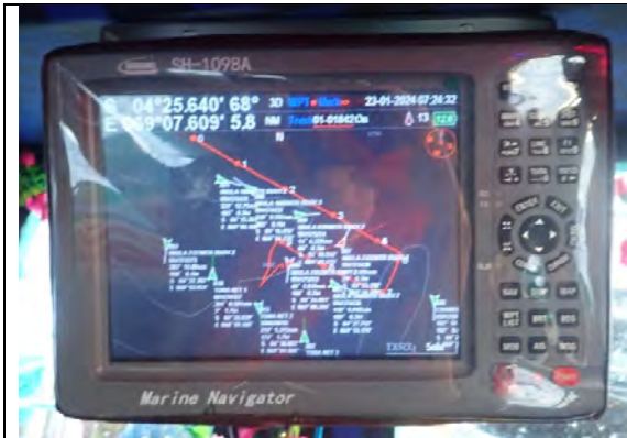
[Fig.7].GPS with AIS tracker and position of the gear
