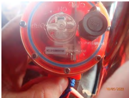
[Fig. 21] Skynav AT-102 AIS GPS tracker, ref number SHO98509150.
