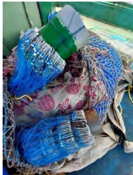
[Fig. 17] Racked snood lines attached to main haul line
