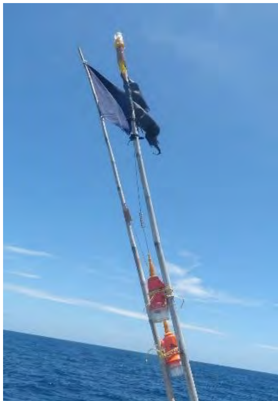
[Fig.24] Dan buoys with mounted AIS transponders
