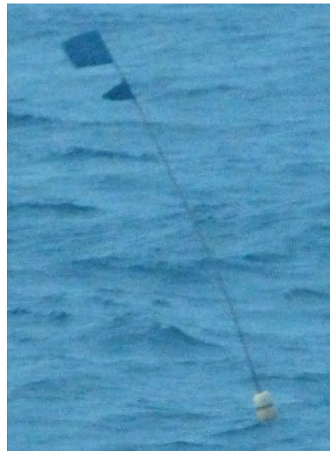
[Fig.35] Final dan-buoy on deployed line.
