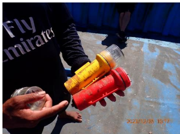
[Fig. 24] Cosmo 2 and 3 used in dan buoys.
