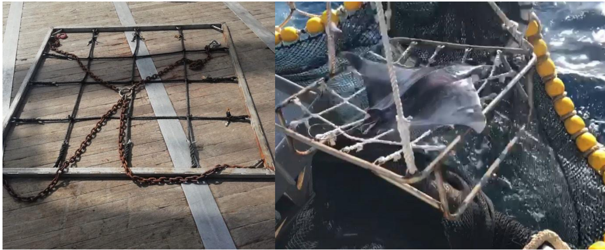
Figure 1. Sorting grid (left) and a mobulid released using the sorting grid (right).
