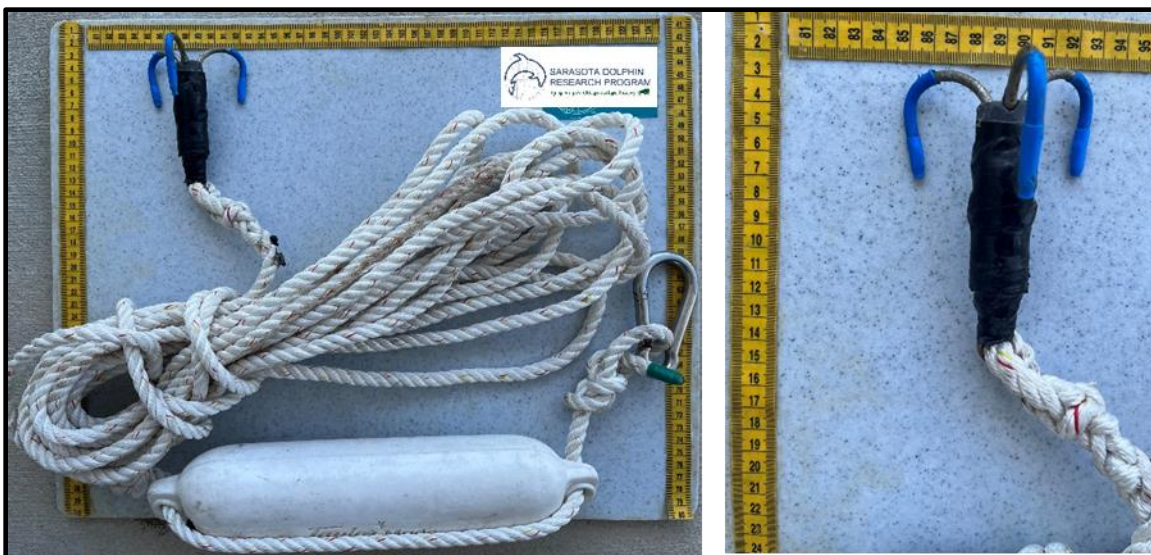
Figure 5. Long-handled grapples with protected tips to avoid injury to the animal.
