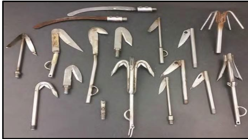
Figure 4. Cutting grapples that can be attached to ropes or poles and extended from the deck of a boat to cut entangling gear. Photo supplied by the Center for Coastal Studies ( https://coastalstudies.org/ ).
