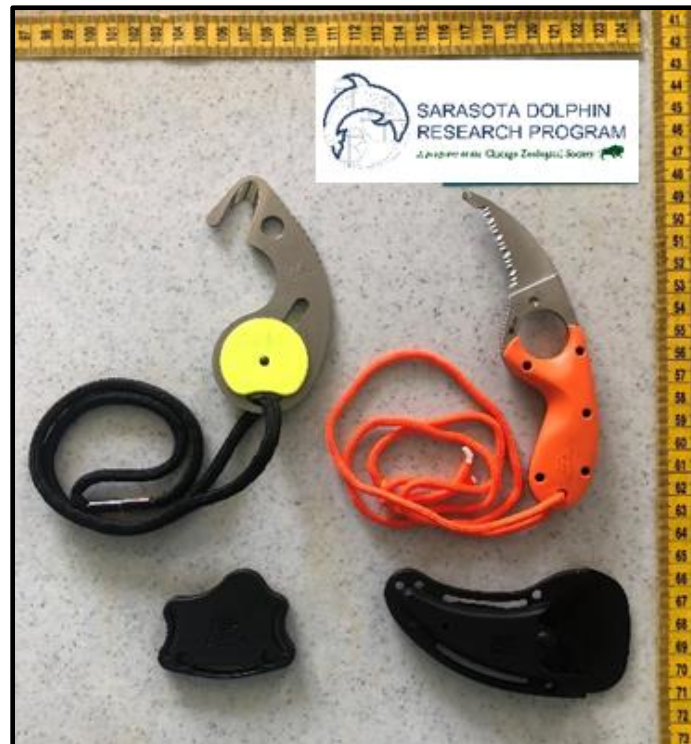
Figure 6. Hand-held cutting tools that can be used in case the animal is brought along side the boat, or lines need to be cut on the boat to prevent injury or accident.
