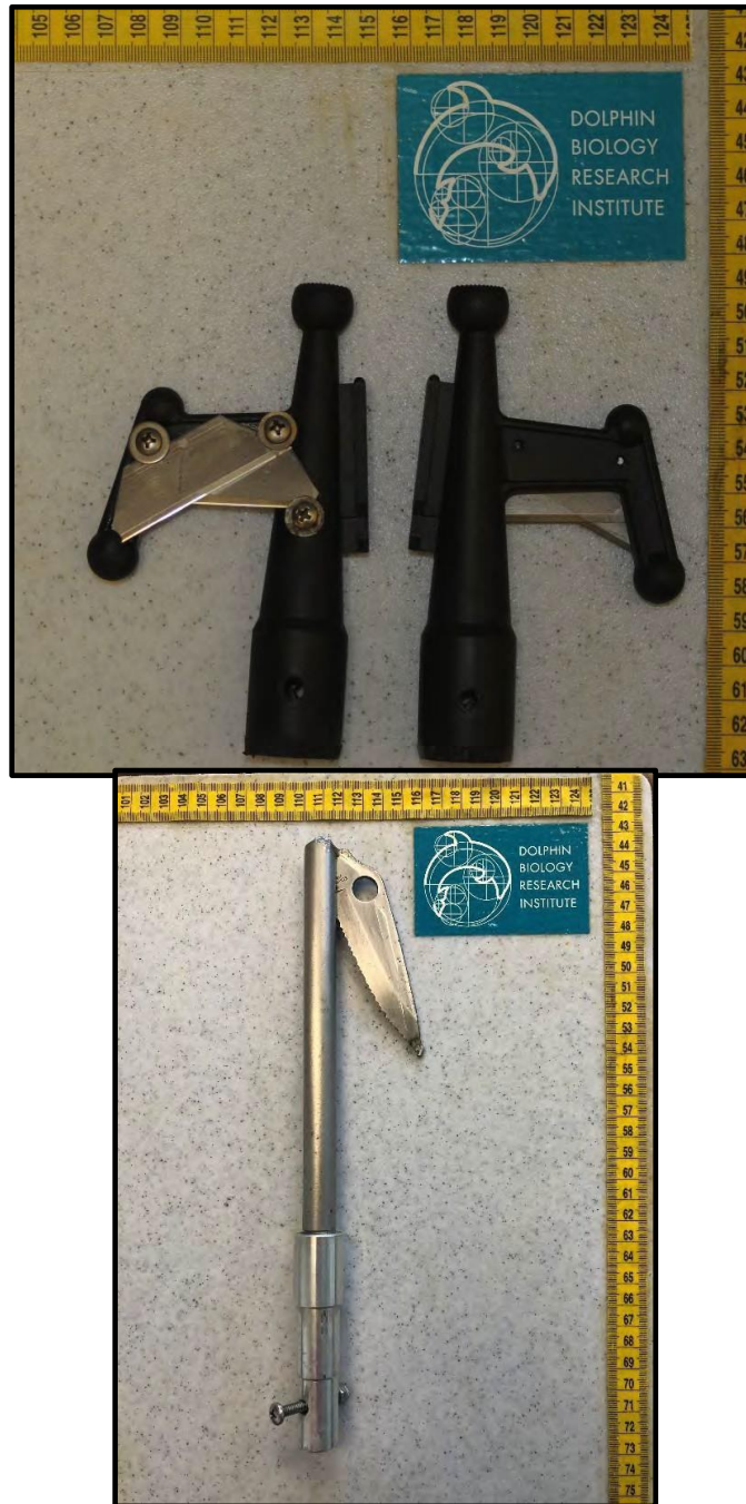
Figure 3. Specially designed cutting tools that can be fitted to the ends of long poles for use from the bow of a boat (Top photo courtesy of the Sarasota Dolphin Research Program, bottom tool designed by the Center for Coastal Studies).
