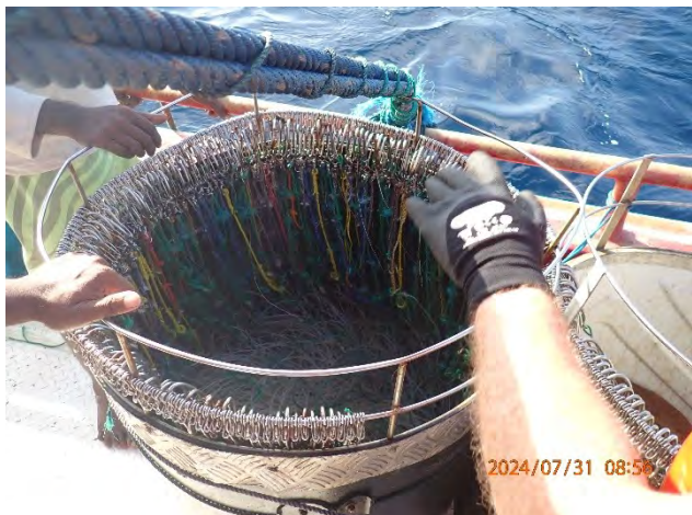
[Fig. 45] Drum with hooks on wire trace, half full.
