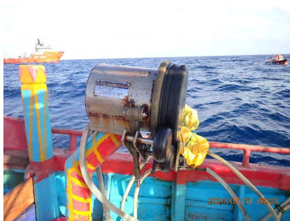
[Fig. 50] A.R.K. Engineering longline hauler/tuna winch.
