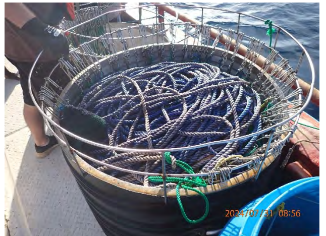
[Fig. 44] Drum with rope and grapples.
