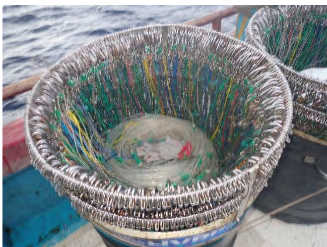
[Fig. 49] Filled drum 1 with hooks (400) on wire trace.
