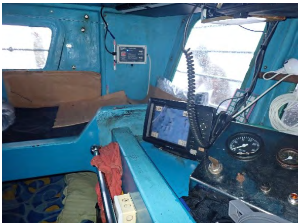
[Fig. 33] Bridge with VMS tracker and plotter, pos. 07°40'S 71°26'E.
