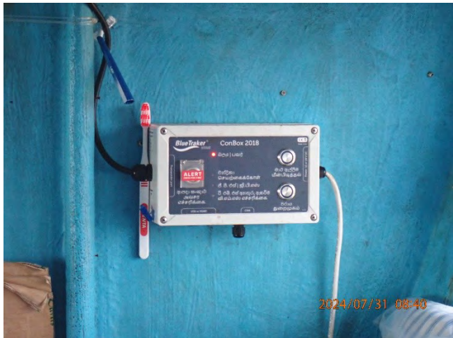
[Fig. 31] VMS system. Blue Tracker Con Box 2018.
