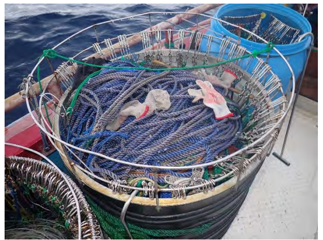
[Fig. 54] Drum with grapples and rope for the longline.
