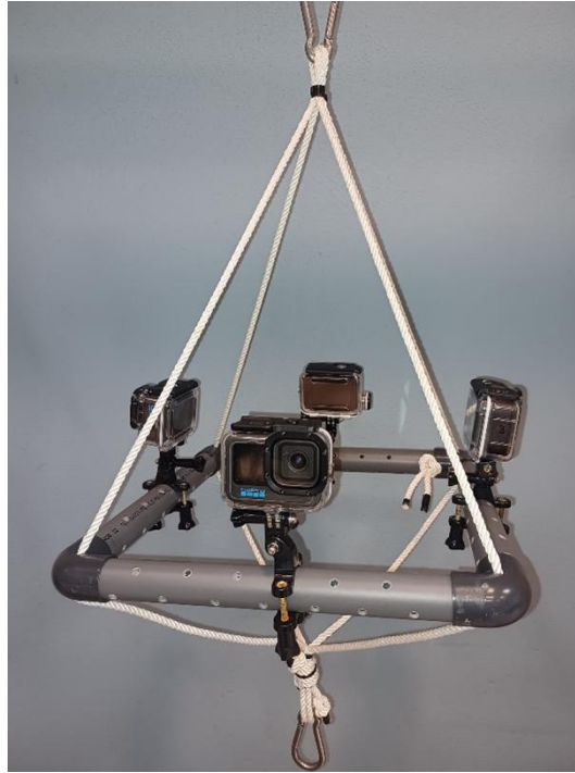
Figure 1. Gadget used for underwater data collection
