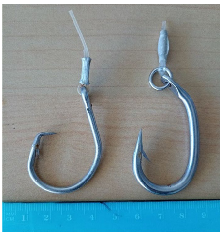
Fig. 1 Hook types used during the experiments: Circle hook (on the left) used in the Gulf of Lions, Japanese tuna hook (on the right) used in Corsica
