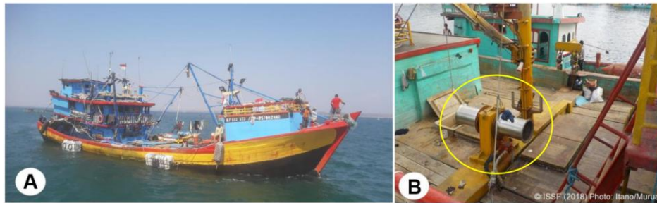
Figure 1a. Illustration a typical purse seine boat (A), equipped with a simple auxiliary fishing device, the horizontal capstan (locally known as gardan) (B), which is used to haul the purse line during net hauling process. The capstan is powered by an electro-hydraulic system, and the nets employed on this type of boat generally range from 600 to 800 meters in length.
