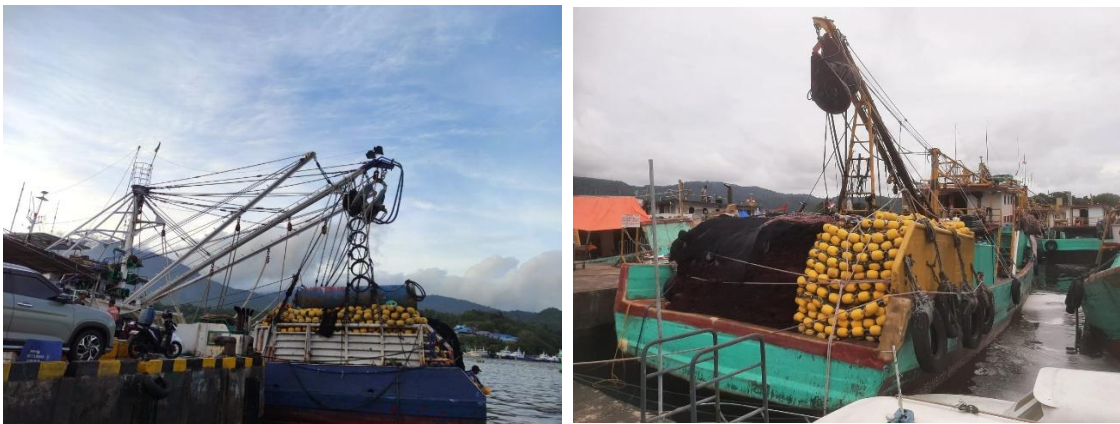
Figure 1b. A typical Indonesian purse seine boat equipped with an advanced auxiliary fishing device, namely a power block, which functions to haul the purse line during net hauling process. The machine is powered by a hydraulic system, and the net length is greater than 1,000 meters.
